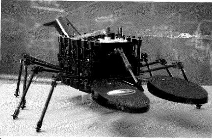
Robolobster, an underwater robot crustacean with eight plastic legs, fiberoptic antennae, and an industrial-strength plastic shell, is remarkably similar to a living lobster in both its form and the manner in which it behaves. Invented by Dr. Joseph Ayers, a marine biologist and neuroscientist at the Marine Science Center at Northeastern University, it was developed in collaboration with Massa Products Corporation, an innovator in electro-acoustic products.
