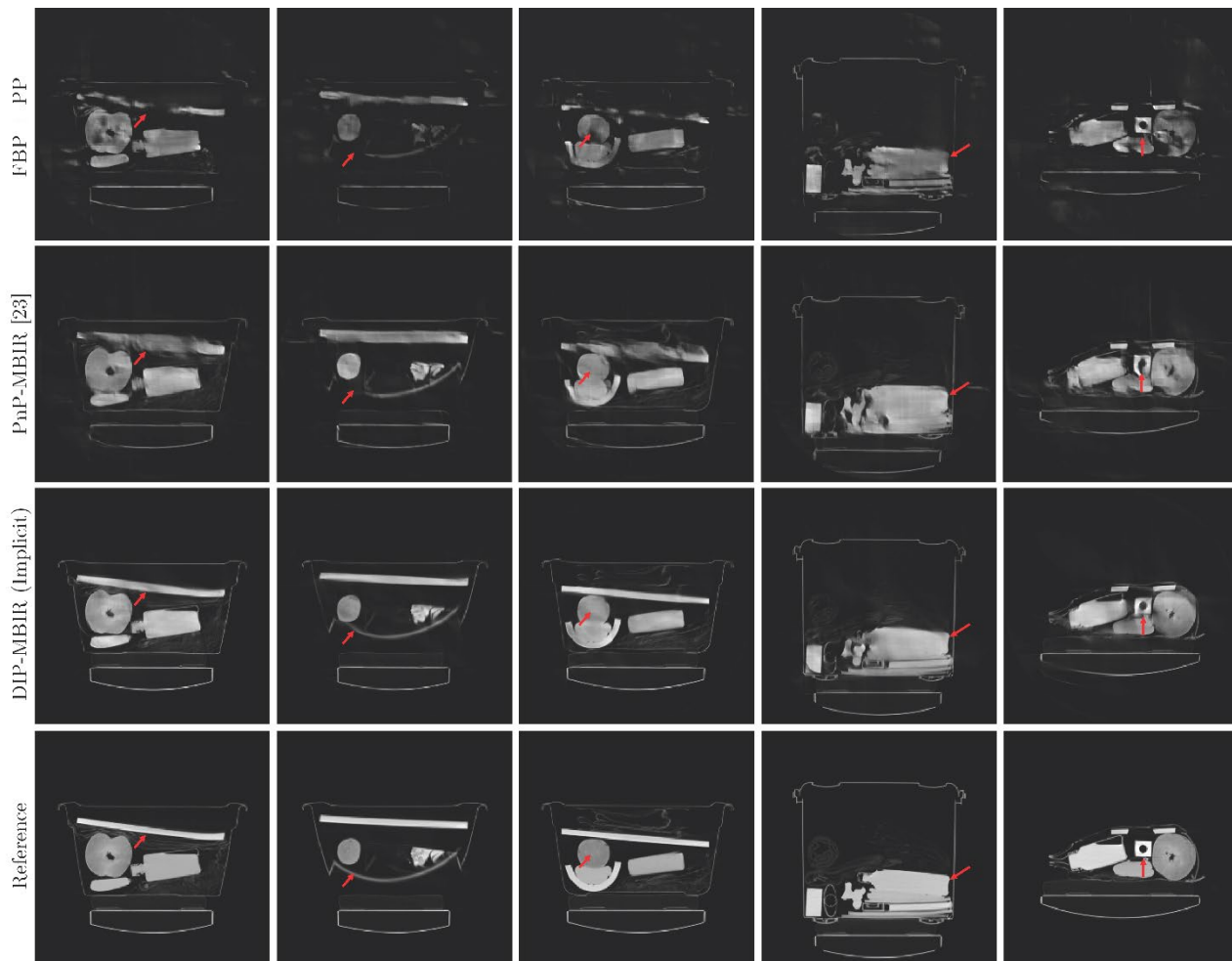
Figure 12: (top row) State-of-the-art deep-learning post-processing and (second row) model-based reconstruction compared to (third row) the new integrated consensus equilibrium-based deep-learning framework and (bottom row) ground truth for a challenging limited-angle tomographic reconstruction problem.
