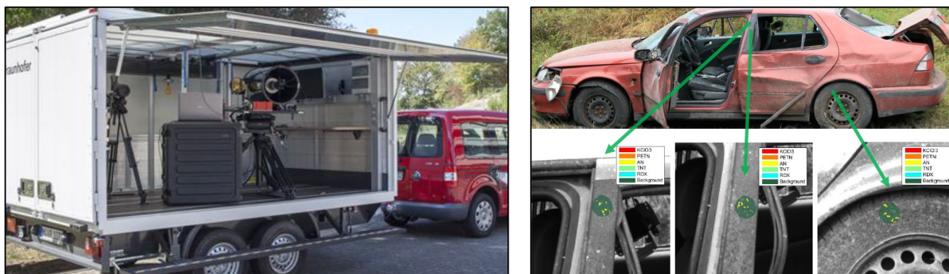
Figure 2: Demonstration of standoff explosive residue detection from [6]. Left, image of trailer platform. Right, detection of AIN residue (yellow marks) after an improvised-explosive-device blast.
