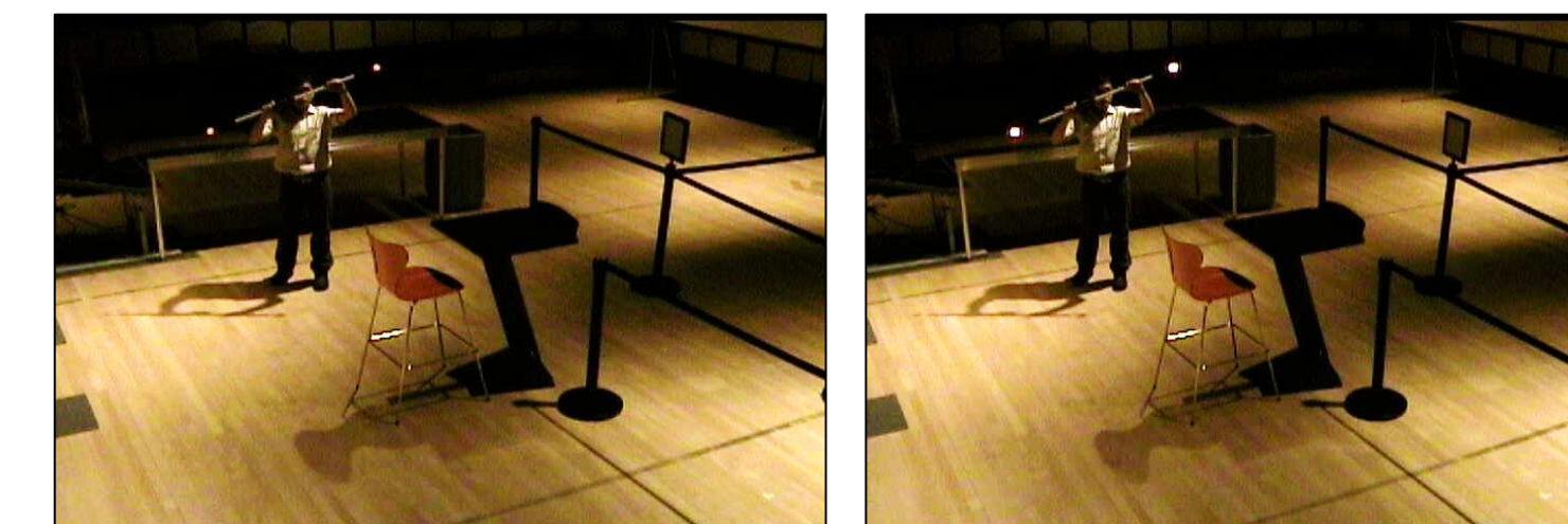
Calibration image with scale bar LEDs on and off.
