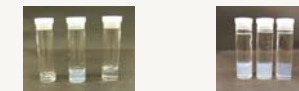
Figure 3: NC alcogels by partial evaporation (left) and by hexane precipitation (right). In both sets, the gels are derived from nitrocellulose solutions containing ethanol, 2-propanol, and 1-butanol solutions, from left to right.
