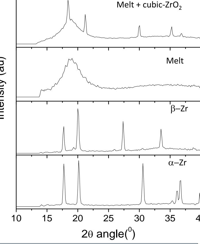
$\alpha$ -Zr initially transforms into  $\beta$ -phase, then melts within 50-60  $\mu$ s
