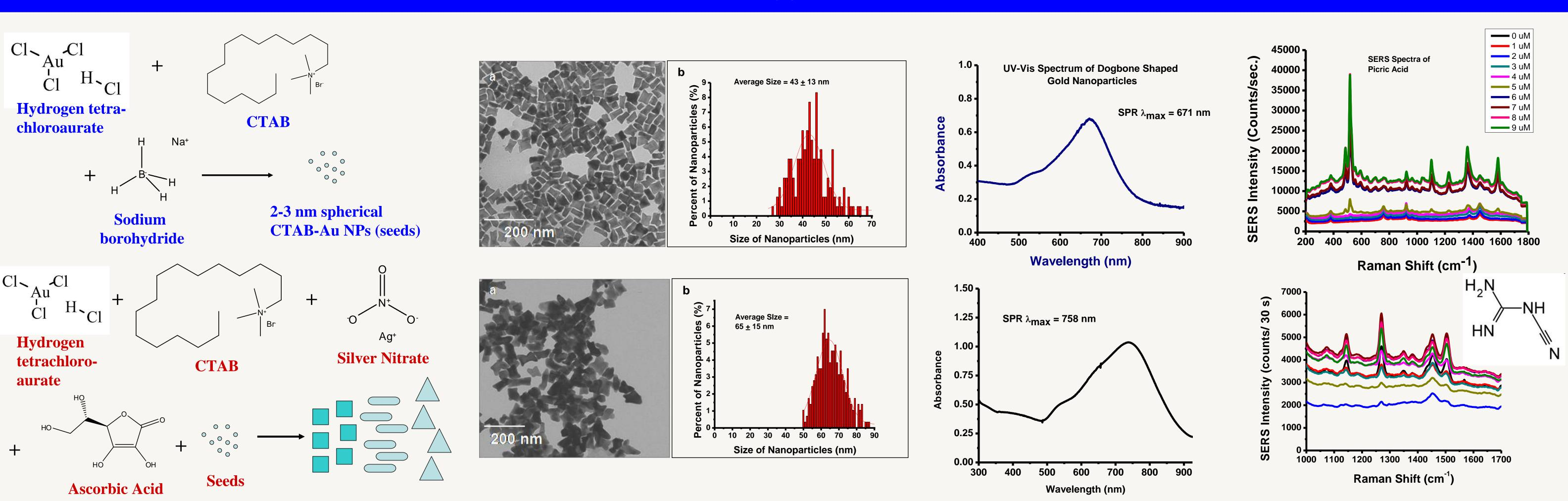
SERS has been used for detection of TNT and DNT vapors adsorbed as thin films in gold substrates. SERS has not been used as a quantitative analytical tool for detection of ultra-low levels of explosives such as dicyanodiamide, methylnitroguanidine, and picric acid. We are using gold nanoparticles of different shapes as colloidal SERS substrates for detection of ultra-low levels of dicyanodiamide, methylnitroguanidine, and picric acid in solution.
