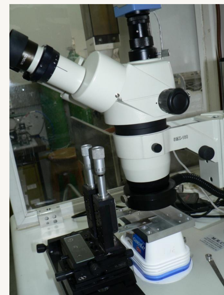
Fig. 1: Device used to glue particles to the cantilever.
