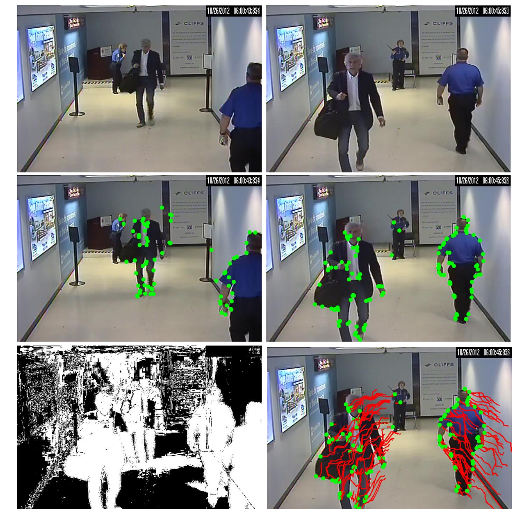
Fig.3 First row: 2 consecutive frames. Middle row: Feature points detection in green. Last row, from left: Motion mask, feature points trajectories shown in red.
