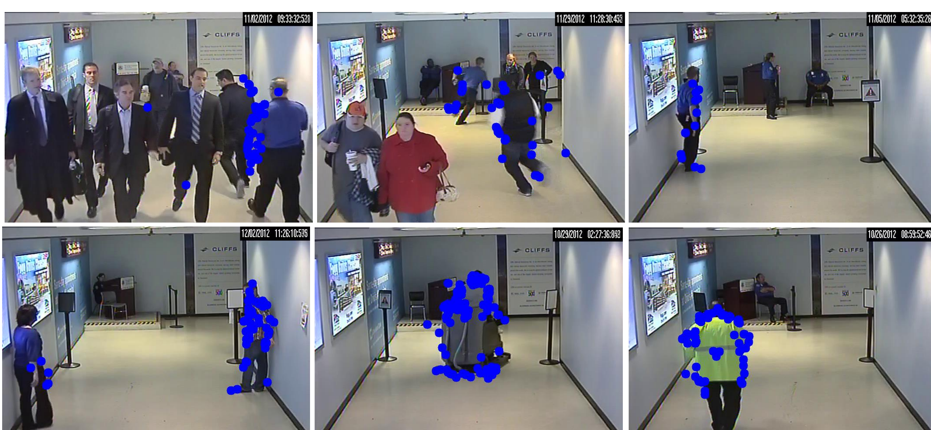
Fig.5 Counter-flow events detected by our technique shown in blue. From top left, in clockwise direction, we have: strong occlusion, fast motion with occlusion, slow motion of 1 person, slow motion of 2 people, an oversized object and a person with a bright coloured jacket.
