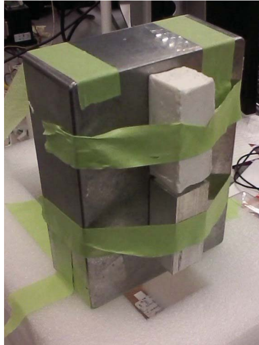
Figure 1: Target object consisting of a flat metal surface with a square metallic and a square dielectric anomaly.
