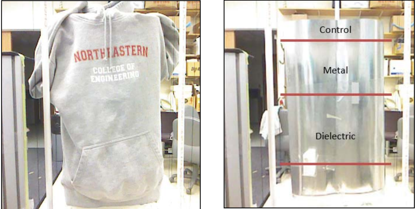
Figure 5: Torso simulant with metal and dielectric explosive simulants.
