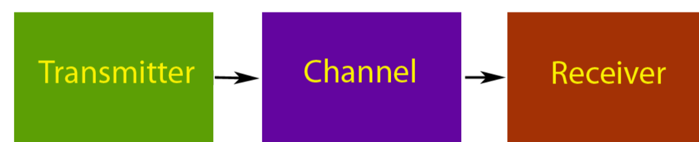
Figure 2: Three parts of a communication system
