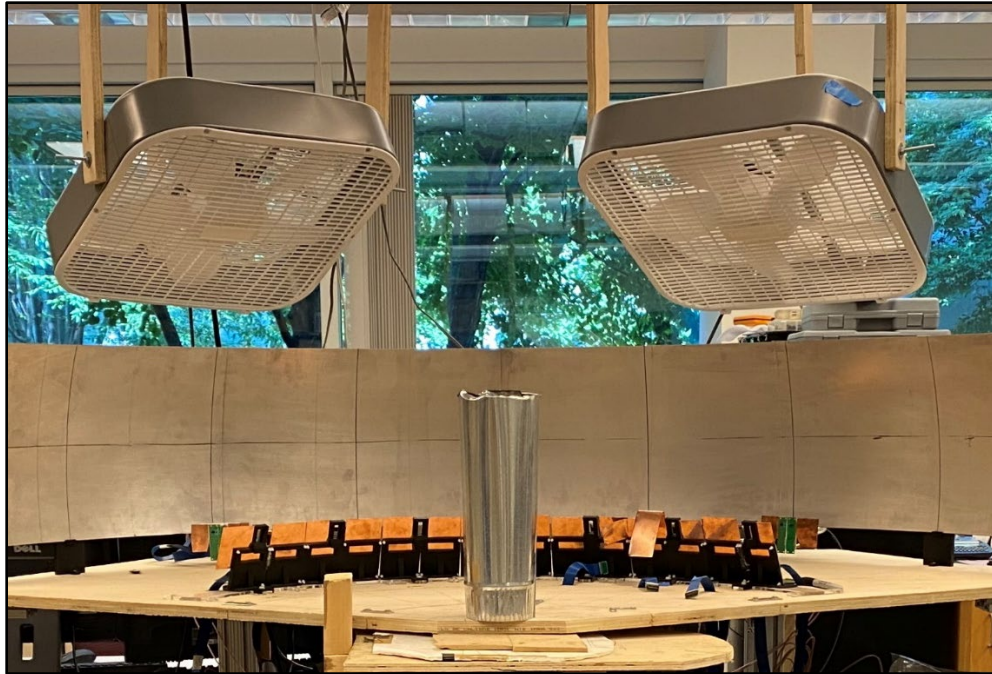
Figure 3: Elliptical reflector antenna with transmitters and receivers (orange) cooled by large fans. A metallic air duct cylinder body part surrogate target is positioned in the target region.
