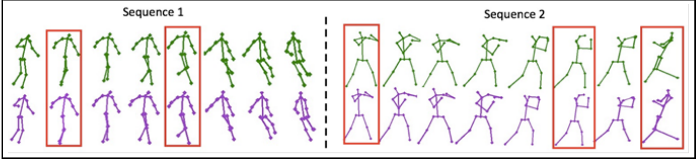
Figure 6: Two examples of the output of our pipeline, (top) ground truth and (bottom) poses recovered from the automatically selected key frames (red boxes).
