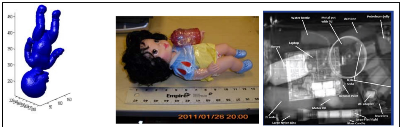
Figure 2-2: (left) Segmented image of (center) doll extracted from (right) CT image dataset of luggage.
